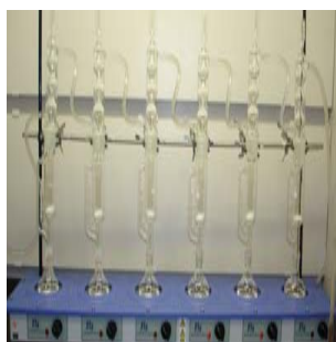
Figure 2: Soxhlet Solvent Extraction Apparatus
